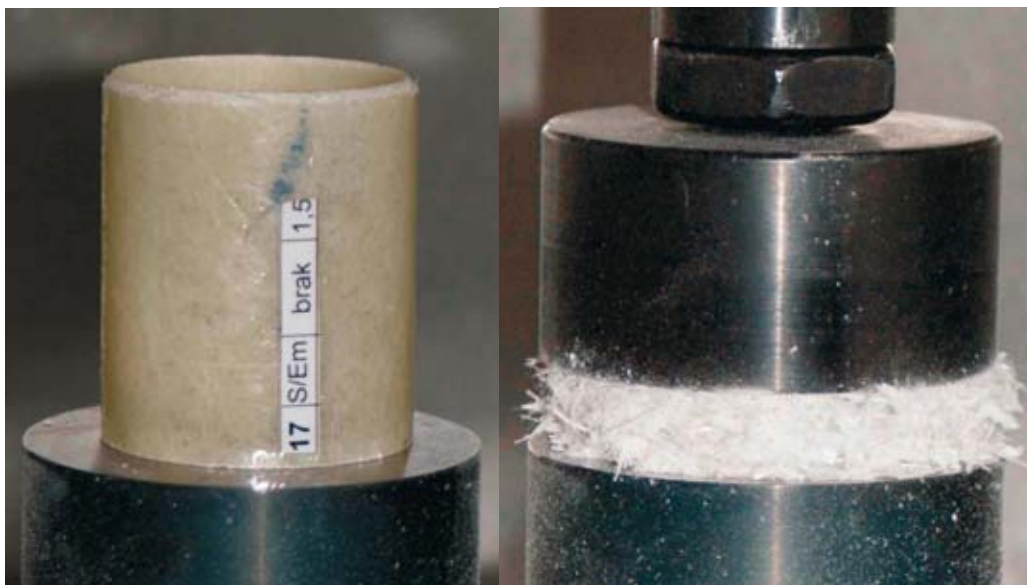
Fig. 3. Composite sleeve after and post impact test
