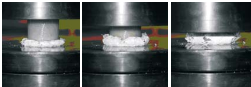
Fig. 1. Failure mode of the composite sleeve
